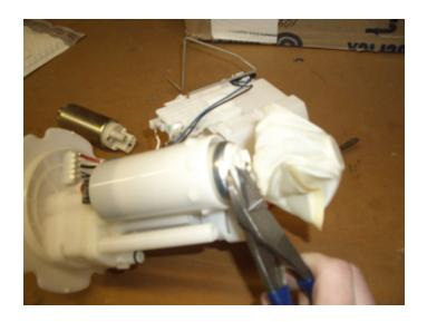
Pump with 3 tabs removed.
