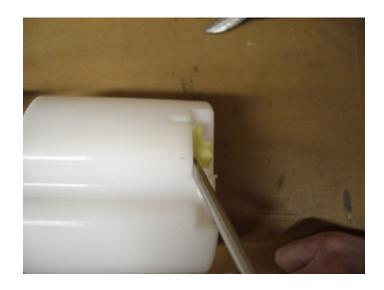
Drill the outlet to .070". If you are using a larger pump like the DW or the Aeromotive, a .100" might be a better idea. Its very soft plastic and drills easy, be careful not to drill all the way through the entire part or it is ruined and not replaceable. Just drill until you can look into the large opening and see the drill has made it to the chamber.
