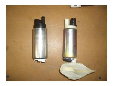
Swap the top seal to the Walbro (Right arrow). Remove the sock by focusing on removing the round metal lock (left arrow).
