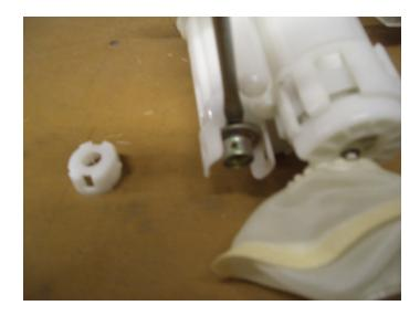
Using a 7/64 drill bit, open the regulator outlet oriface. ONLY drill until you make it thru the sheet metal.
