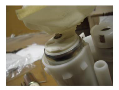
Mark this part of the pump cap to file off. Notice the green marking.
