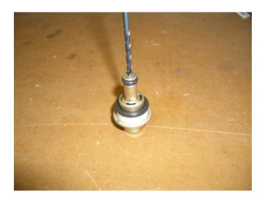
Blow the regulator off with compressed air. Making sure both o-rings and the plastic spacer are in place, reinsert the regulator into the housing and reinstall the regulator cap.
