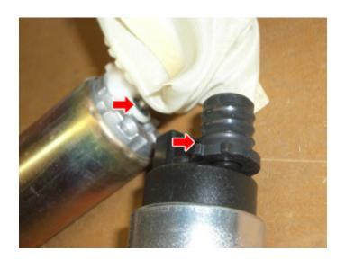
Put the sock on the Walbro, and put the metal lock on the Walbro. Be careful, the metal lock is hard to get back on, and very easy to loose if it gets away on you.
