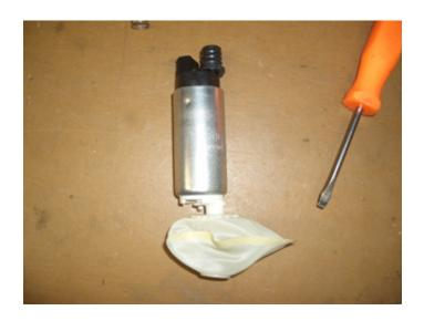
Slide the Walbro back into the assembly. Make sure you feel the top seal slide into its position. Plug back in the electrical connector.
