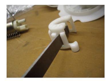
With some muscle, starting on the left and working your way to the right, reinstall the pump cap onto all the locks. It can be done at this point but if you feel that you just cannot get it to snap and lock SECURELY on, you can file other sections down to allow more room. Just be careful, if you file too much then the pump will fit loosely, you want it extremely snug and you want to make sure the cap is correctly seated so that it does not pop off. It should be flexing just a little to get on.
