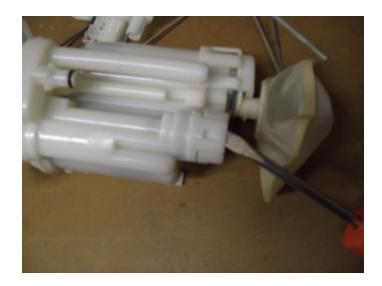
Remove the regulator. Just put a screwdriver under the lip and twist, it pops out easy.
